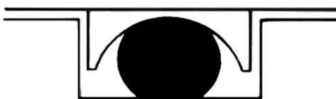
Installed O-ring energized sealing element (no system pressure)
