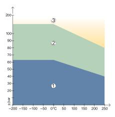
KLINGER Hot and Cold Compression Test Method The KLINGER Hot Compression Test was developed by KLINGER as a method to test the load bearing capabilities of gasket materials under hot and cold conditions.
