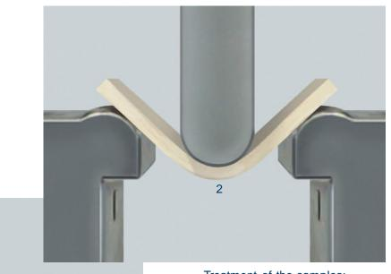
Treatment of the samples: 48h at 200°C 1. Standard fibre reinforced material 2. KLINGER<sup>®</sup>Quantum Flexibility at High Temperatures The 3-point bending test is often used as an evaluation method for the flexibility of fibre-reinforced gasket materials. Special tests on conditioned specimens provide an indication of the brittleness and hence of the aging behaviour of the elastomers used.
