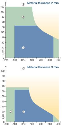
As the maximum operating pressure and load bearing capability are both depending on the gasket thickness, KLINGER provides thickness related pT diagrams.
