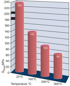
Creep relaxation factor  $P_{QR}$ acc. to EN 13555 This factor considers the relaxation influence on the gasket load between the tightening of the bolts and the long-term effect of the service temperature.
