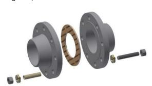
Figure 1 – Typical assembly with GW1 washers
