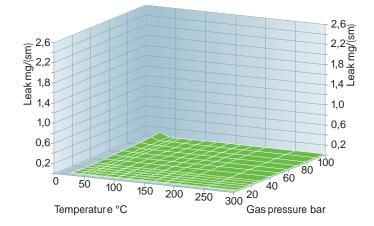
Stabilisation time for each reading is two hours and a new test specimen is used for every gasket load and temperature.
