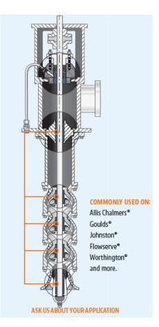
OEM bushings are supplied of many materials with normal clearances of .015" to .020". These materials tend to wear rapidly, the clearances open, and the shaft is no longer steadied.
