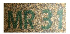
MR 31 Cork is a highly compressible automotive and general purpose gasket material with moderate oil resistance.
